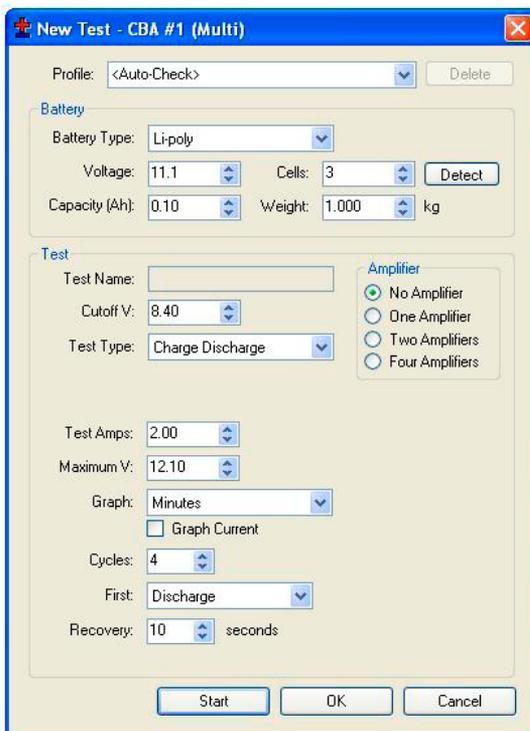
The test alternates between charge and discharge cycles. Discharging is accomplished with a WMR CBA III or CBA IV. Charging is accomplished by having a the WMR CBA Charger Interface board control an off-the-shelf charging unit that the customer will provide. When using Charge/Discharge test the software will disable the "Test Name" field. Instead the software will create test names 'Charge n' and 'Discharge n' automatically (where n is the cycle number, and increments automatically).
