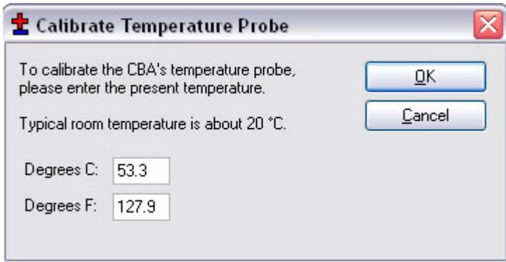
In the standard version of the software the temperature is displayed and the temperature may be used as a safety feature to automatically stop a test at a user set maximum battery temperature.
